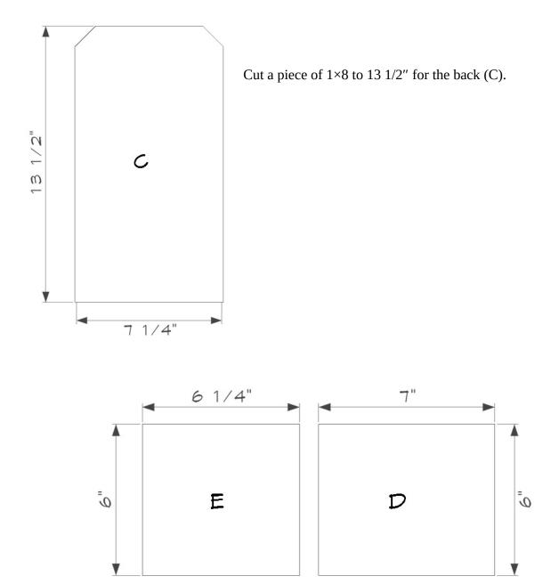
Cut one piece of  $1 \times 8$  to  $6'' \ge 6 1/4''$  (E), cut one piece to  $6'' \ge 7''$  (D) for the roof.
