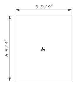
Cut a piece of  $1 \times 8$  to  $5 3/4'' \ge 6 3/4''$  for the floor (A).
