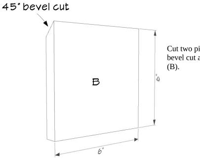
Cut two pieces of 1×8 to 6" x 6", cut a 45-degree bevel cut as shown on drawing above for the sides (B).
