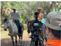
You should use a tripod when conducting interviews. Notice the "shotgun" microphone on the video camera.
